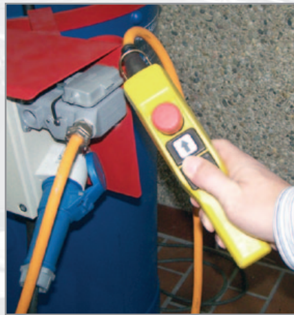
Button control, pluggable, for assembly and operation control.
