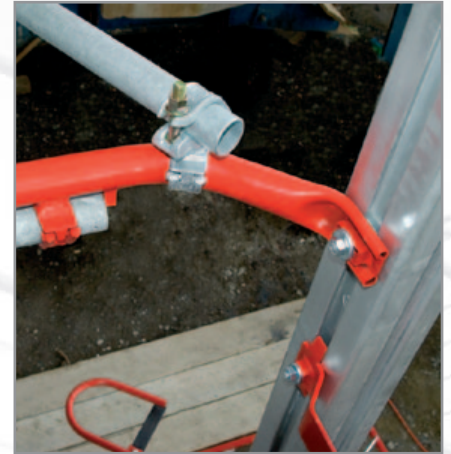
Mast fixing – The aluminium mast can be steplessly fixed to the scaffold resp. building.
