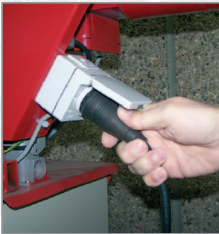
230 Volt socket on the carriage to operate assembly tools.
