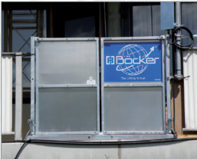
Landing gate complies with machinery directive 2006/42/EG
