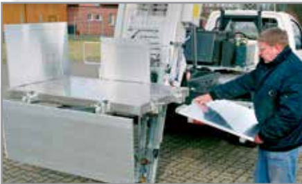
Side panels foldable 90° / 180° and completely removable
