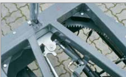
Infinitely variable, hydraulically releasable live ring lock
