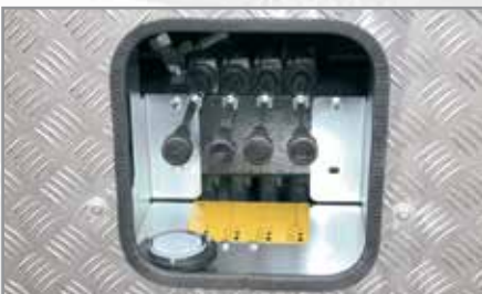
Control stand for hydraulic supports
