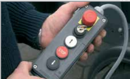
Electric control via cable operation
