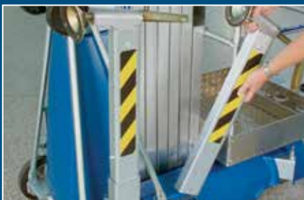
7 Outrigger brackets facilitate the transport
